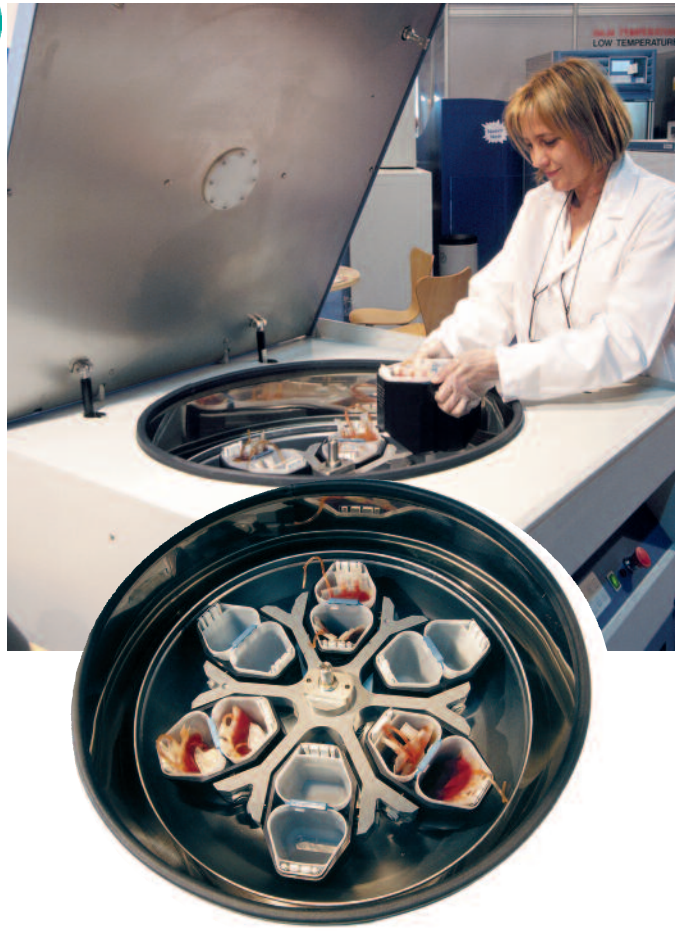
Image showing the rotor and double buckets for quad and triple blood bags of 500 and 800 ml.
