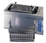
Racks: made of AISI 304 stainless steel.
