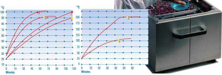
Graph of temperature and time for the Tectron Bio 100 and Digiterm-S-100 and Digiterm-TFT-200, units with capacity of 20 litres.
