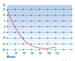
Graph showing the cooling performance of the 8 litre  $H_2 O$ "Frigedor" With insulated stirring tank.
