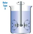
**Radial flow**, diagram showing the agitation within the liquid. Representative of radial turbine rotors that run parallel to the stirring axis.
