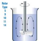
**Axial flow**, diagram showing the agitation flow. Representative of rotors with blades angles of 90° in relation to the stirring axis. (Rotor type; Helix).
