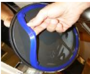
Fig. 7.3 Door gasket replacing.
