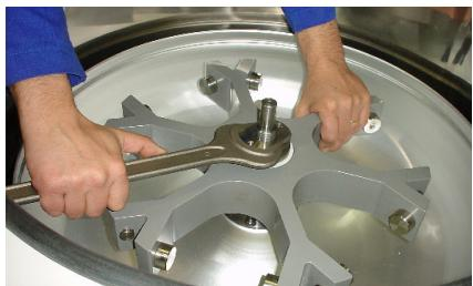
Place and screw the locking nut in place and tighten using the spanner provided.
