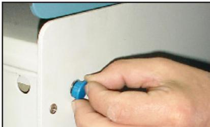
Once the unit is installed, remove the lifting supports and put the hole taps supplied into place.
