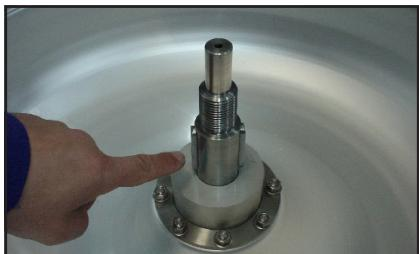
Before placing the swing out rotor, check that the locking ring wedge is in the right position.
