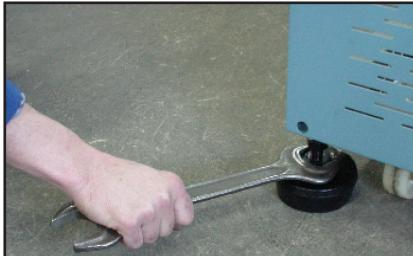
Adjust the 4 levelling rubber feet supports so that the unit is raised and do not rest on the wheels, and adjust until the machine is levelled.
