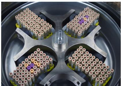
Periodically examine the status of the rotor and the buckets to check and detect possible corrosion, micro fractures and mechanical deformations.
