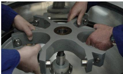
Place the rotor on the spindle, ensuring that the keys and their lodgings are perfectly aligned and that it fits perpendicular to the axis. The rotor should slide easily, **it is not necessary to use a mallet or hammer.**
