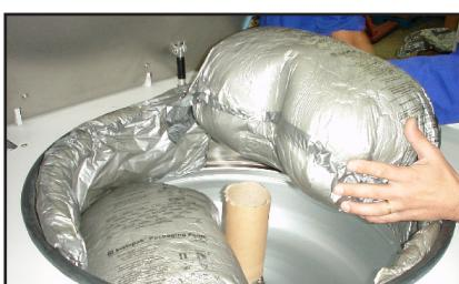
Remove the packaging protections from inside the chamber. Check that there is no packing material remaining in the unit.
