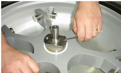
Tighten the Allen screws on the locking nut block.
