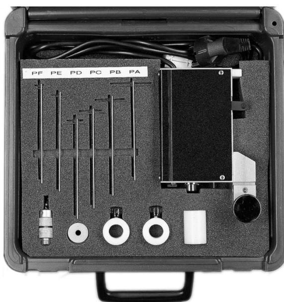
Fig. 15 Kjeldahl Unit in its case
