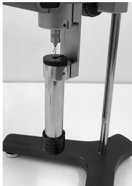
Fig. 8: LCP Adapter assembled in viscometer
