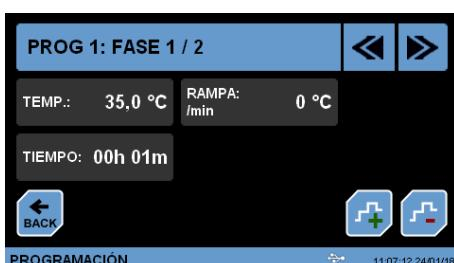
Fig. 8.4.1 Modify temperature, ramp and time parameters.
