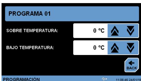
Fig. 8.4.2 Modify maximum and minimum temperature limits.
