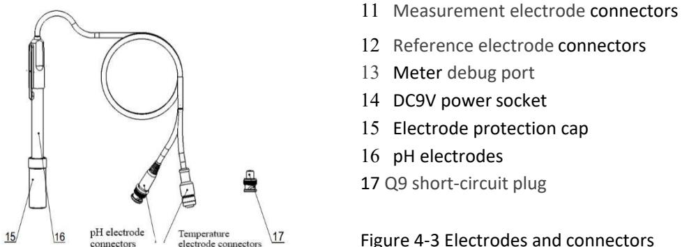
Figure 4-3 Electrodes and connectors
