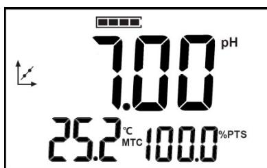
Figure 5-7 Calibration display
