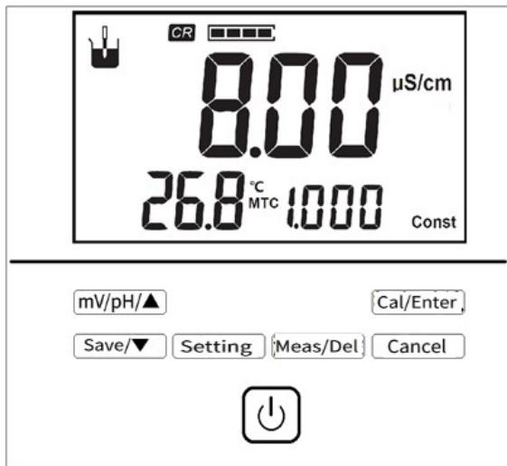
Figure 5-2 Instrument keys
