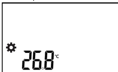
Figure 5-5 Setting temperature value display
